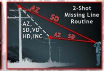
TruTargeting: This automatically provides the best possible accuracy and acquisition distance to a given target. If the displayed measurement has a decimal value, you are getting the +/-1 ft (30 cm) accuracy. If a whole number is displayed, your accuracy is within +/- 1 yd (1 m)
